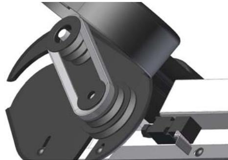
Img.3-8: Assembly V-belt
