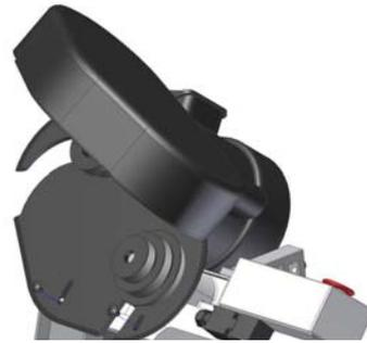
Img.3-7: Assembly V-belt housing
